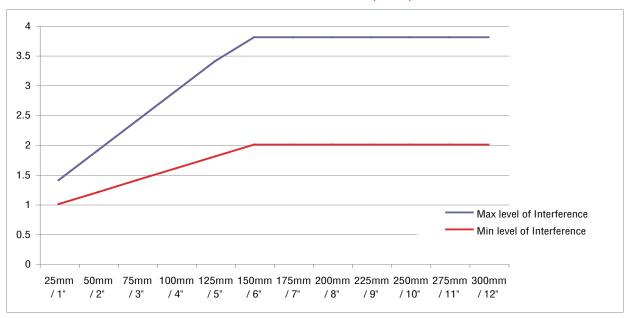
Eg - The spring lip measures 48.5mm and does not appear to be heavily worn, the shaft diameter would be between 49.6mm and 50.3mm (48.5 + 1.1 = 49.6, 48.5 + 1.8 = 50.3). Shaft size is most likely 50mm.
