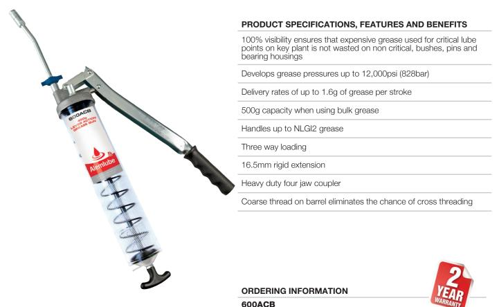
450g Clear Barrel Lever Action Grease Gun
