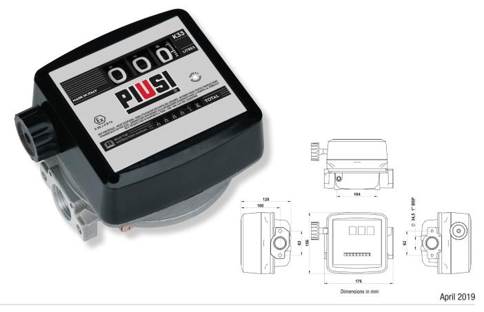
The 51008P mechanical petrol meter has an aluminium body incorporating an inlet and outlet threaded flange and can meter petrol varieties ULP, E2O, aviation fuel (Avgas), kerosene and diesel accurately between 20 L/min & 120 L/min and is thus ideal for applications in hazardous environments due to its ATEX / IECEx approvals.
