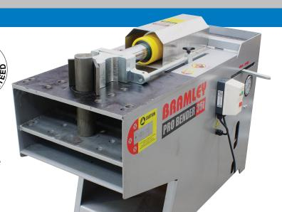
The standard machine is a robust powered hydraulic bender of 35 tonne rated capacity supplied with attachment for bending flat bar up to 100 x 12 mm or round & square bar up to 25mm
