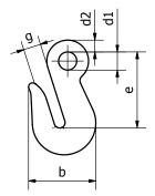
Used for the shortening of chain sling legs. It's the first grab hook in Grade 100 on the market. Due to its unique design there is no deration in the load capacity. This is due to the 4 fold feature of the hooks supporting cradle design.
