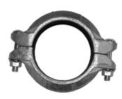
Application: Transition couplings are designed to join 150mm Australian Standard Pipe OD 165.1mm to 150mm American Line Pipe OD 168.3mm.
