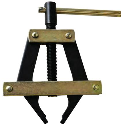
Tip: To avoid unnecessary bending of link plates, press pins out evenly. Pop the rivet of the first pin and then the second, when both pins have been 'cracked', proceed with fully pushing the pins out.
