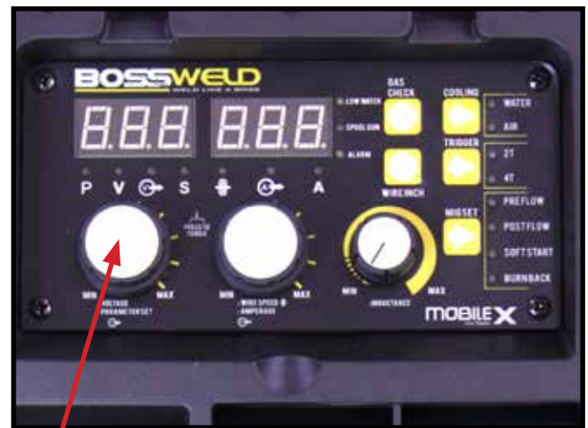
13 To adjust welding voltage, turn the voltage adjustment dial on the SWF.
