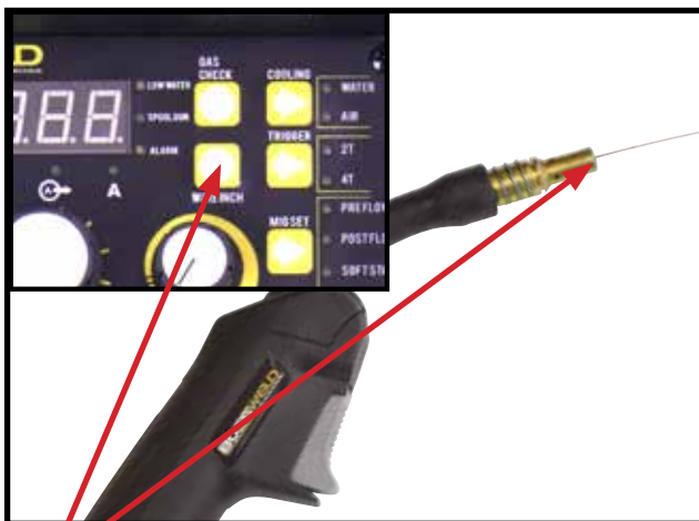
10 Remove nozzle and tip from torch and press inch feeding button, this will feed the wire through the torch. Release button when wire appears at the end of the torch.
