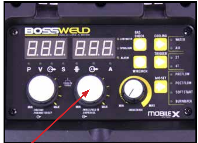
15 It is recommended for ease of use that the wire-feed target speed is adjusted first and then the voltage setting fine-tuned if necessary. To adjust wire speed, turn Welding parameter Adjustment Knob. Ref MIG Welding Setting Guide on page 33-34
