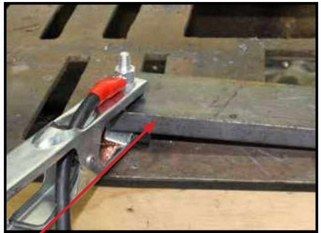
14 Connect earth clamp to the work piece ensuring that the clamp makes good contact with bare metal.
