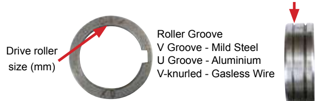
5 Remove the Drive Roller Covers. Check the Drive rollers are matched to the wire size for the job Note: Correct wire side on roller to face into machine when fitting. Then replace the Drive Roller Cover.
