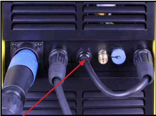
5 Ensure the polarity is correct for gasless welding, DCEN
