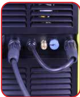
C DCEN Polarity Switching Terminal Set for Gasless Welding
