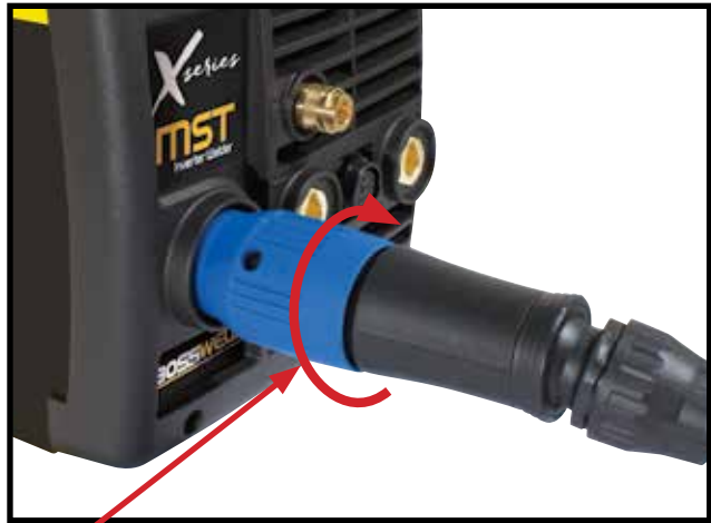
4 Install Euro connect MIG torch over the protruding wire, line up the spring connectors and screw the Euro connector nut up firmly.
