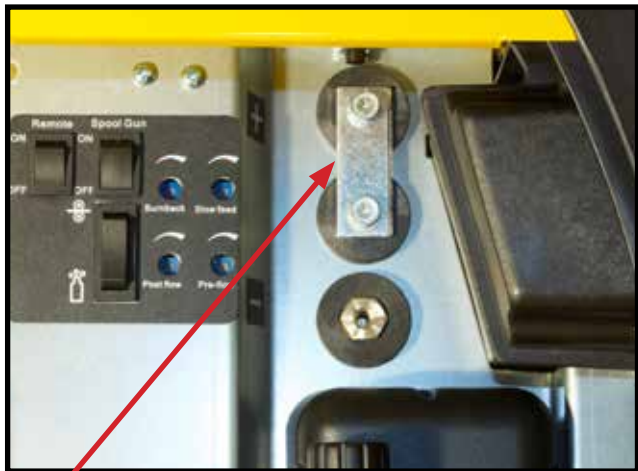
5 Ensure the polarity is correct for gas welding, DCEP
