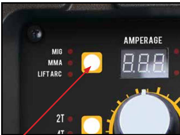
8 Press the Welding Mode Selection Button until the MIG indicator is lit.
