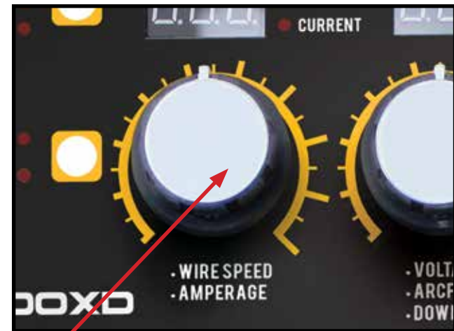
11 It is recommended for ease of use that the wire-feed target speed is adjusted first and then the voltage setting fine-tuned if necessary. To adjust wire speed, turn Welding parameter Adjustment Knob. Ref MIG Welding Setting Guide on page 33-34
