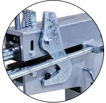
Showing Hook Plates in down position for heavy swaging work.
