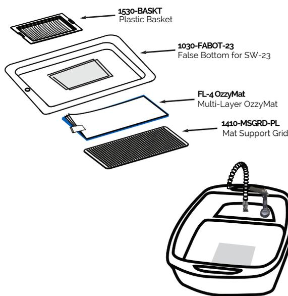
1. Remove the OzzyMat® from its package, unfold it and lay it on the mat support grid located in the lowest level in the sink. Make sure to lay the OzzyMat® white side up.
