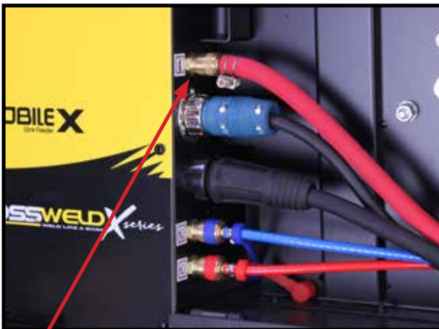
16 Install gas hose from the interconnecting cable to the gas inlet on the back panel of the SWF.
