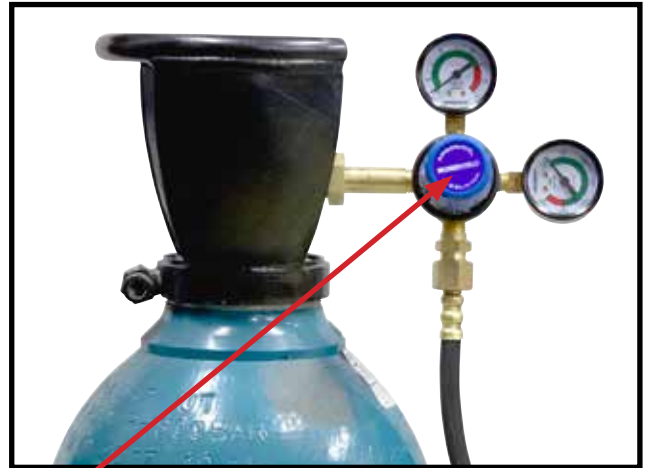
17 Turn on regulator and set gas flow to between 10-15 L/min depending on your welding environment.
