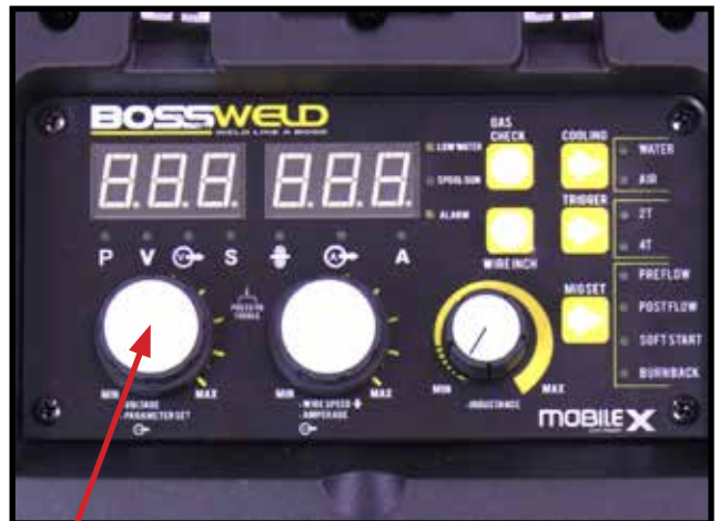
16 To adjust welding voltage, turn Welding parameter Adjustment Knob. Ref MIG Welding Setting Guide on page 38
