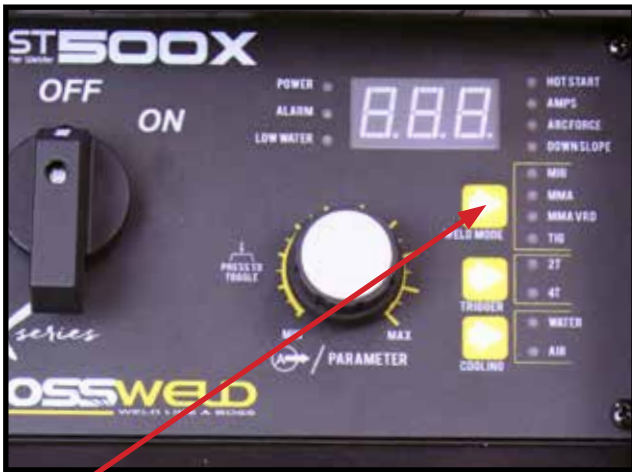
8 Select MIG on power source control panel
