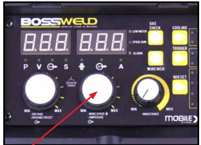
12 It is recommended for ease of use that the wire-feed target speed is adjusted first and then the voltage setting fine-tuned if necessary. To adjust wire speed, Turn the Current dial on the SWF. The digital display on the power source will show the setting selection. Ref MIG Welding Setting Guide on page 38
