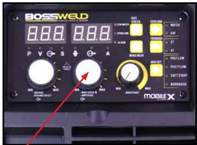
12 It is recommended for ease of use that the wire-feed target speed is adjusted first and then the voltage setting fine-tuned if necessary. To adjust wire speed, Turn the Current dial on the SWF.
