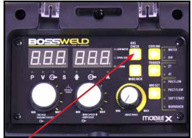
18 Check the gas flow by pressing the gas check button.
