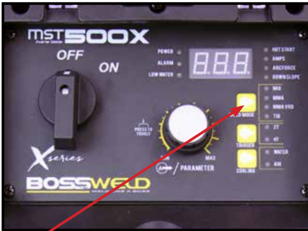
8 Selection switch to MIG on front panel of power source
