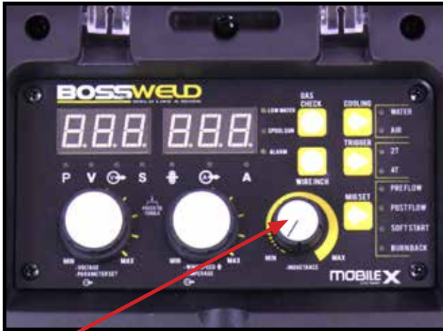
14 To adjust Inductance, turn the inductance dial on power source.
