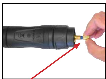
2 Remove the liner retaining nut from the euro torch end.
