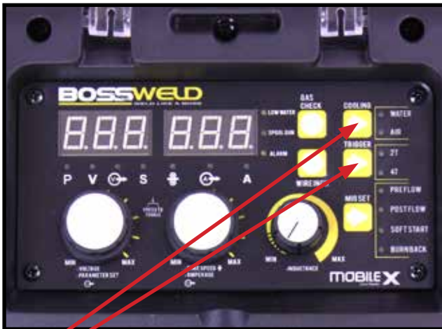
9 On the wire feeder control, select water or air for MIG torch cooling. Only select water if a water cooled MIG torch is installed. Select 2T or 4T trigger mode.
