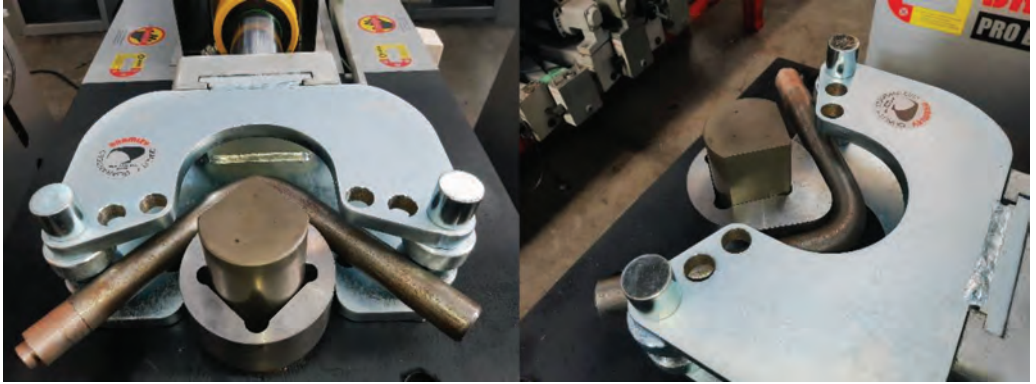
Shown here is 32mm mild steel round bar bent to 90°. Mild steel up to 32mm may be bent using the small radius (except rebar for structural use).
