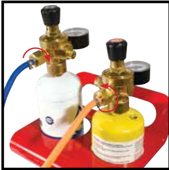
10. Attach the hose to the fuel and oxygen regulators
