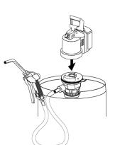
Note: Power head will not oprerate unless locked correctly into position.
