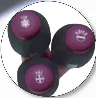
The non-slip handle is made from cellulose acetate and has a micro-fine surface structure. This gives maximum torque transmission and perfect handling in wet and oily work surroundings.
