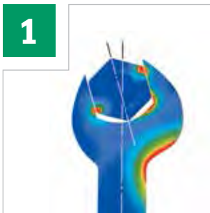
Load zones in standard-quality spanners
