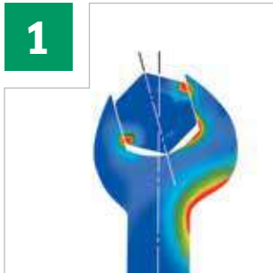
Load zones in standard-quality spanners
