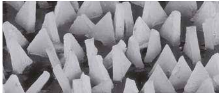
The VICTO GRAIN abrasive grain is optimally aligned
