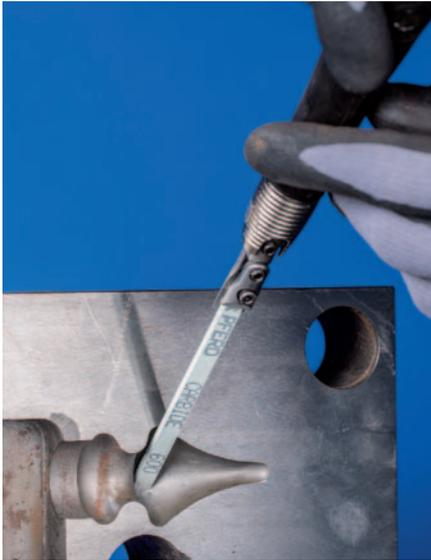
PFERD grinding and polishing stones are versatile tools for finish machining on forms in tool and mould-making. They are used for step-by-step fine grinding after machining or after electrical discharge machining (EDM) to grind in a brushed finish/polish in the demoulding direction or to prepare for high-gloss polishing with diamond pastes.
