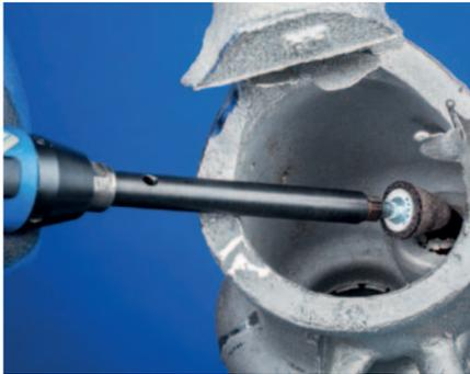
Mounted points with a shank diameter of 3, 6 and 8 mm can be extended with drive spindle extensions. They allow access to hard-to-reach areas. The drive spindle extension is mounted in the collet of the tool drive (air grinder or electric grinder), or in the handpiece of the flexible shaft. In some applications, spindle extensions are an economical alternative to customized mounted points with long shanks.
