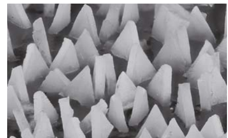
The VICTOGRAIN abrasive grit is optimally aligned
