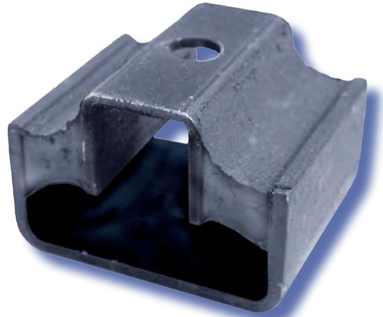
If used as engine supports ( fig 2) the U- Flex isolator should be employed so that maximum flexibility ( X ) is used vertically and ( Y ) at right angles to the crankshaft as the vibrations are most severe in these directions.
