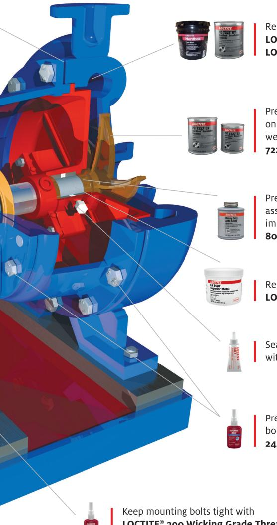
Rebuild and protect worn volutes with LOCTITE<sup>®</sup> PC 7226 Pneu Wear and/or LOCTITE<sup>®</sup> PC 7227 Brushable Ceramic
