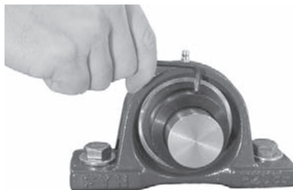
Fig. 14.10 Installing eccentric locking collar
