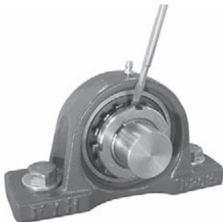
Fig. 14.8 Bending claw of washer (Locking locknut)
