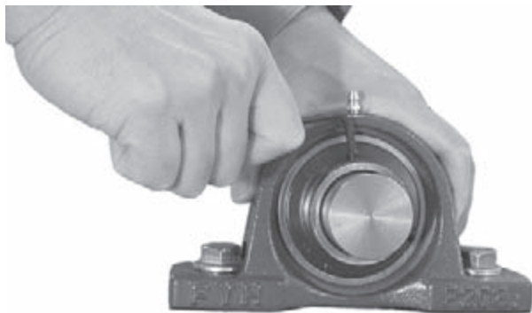
Fig. 14.5 Tightening of set screws
