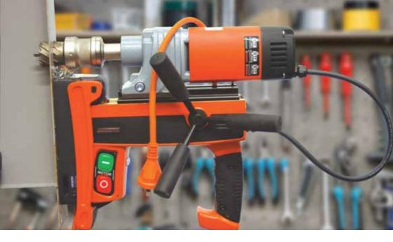
The new, unique Magnex Drill provides improved safety by using a powerful magnet that does not need a power supply to work.
