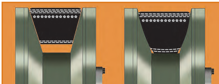
Proper Position of Belt in Sheave
