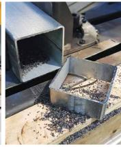
MBR35525465 | 355mm RaiderX Metal blade achieved 3,857 cuts, then professionally sharpened (at a cost of \$30). The blade completed a total of 10,000 cuts - still cutting but leaving a very small burr.
